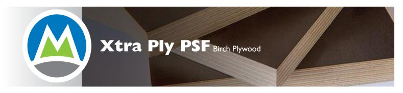
Xtra Ply PSF is a film faced plywood, composed entirely of thin layers of Birch veneers, bonded with exterior phenolic resin adhesive. Each panel is laminated with multiple veneer layers to enhance the structural properties, then sanded uniform and overlaid (both sides) with a dark brown phenolic surface film. Each panel has sealed edges to help minimize moisture absorption.
